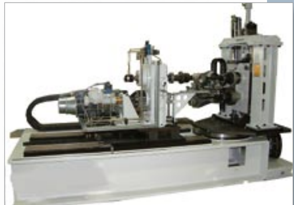
Lateral shaft test stand, hydraulic tension output 400 kW
