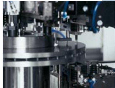
RotaMat D Automatic Measuring and Crack Testing Machine for brake discs and drums
