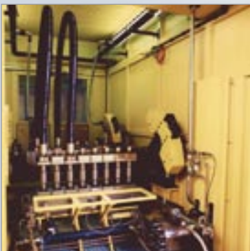
Pressure pulse test stand with mobile unit for flexible hydraulic piping systems
