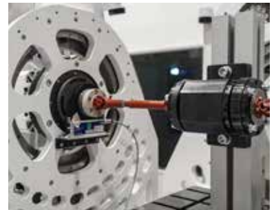
Length compensation with side shafts
