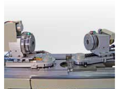
Motor-driven adjustment of the articulation angle for unit left. Manual adjustment of the articulation angle for unit right.
