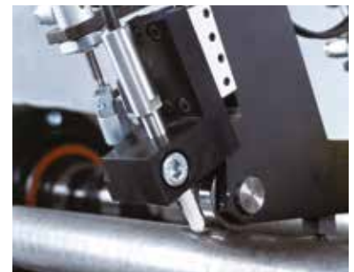
Reliable 100%-testing for surface-breaking damage to drive shafts
