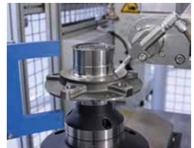
Crack testing of wheel hubs with additional hole counting by means of a light barrier
