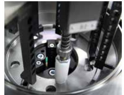
Precise inside measurement of brake drums
