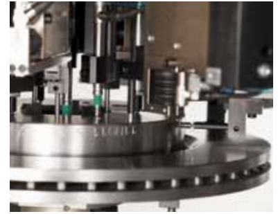
Dynamic measurement with acquisition of all measurement characteristics in a single rotation
