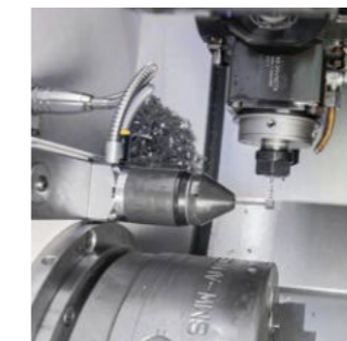
Tool measurement – TC76 with protective sleeve
