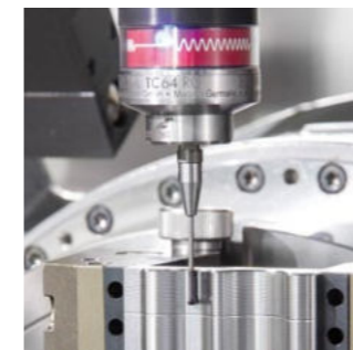
TC64-RG – Roughness measurement in the machining centre
