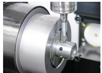
Analogue scan of a conical elongated hole
